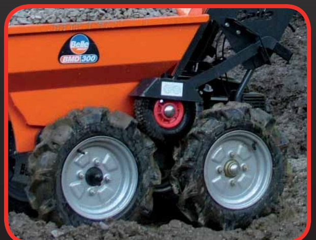
Carrier wheel disengages for easy wheel change
